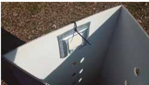
Figure 112. Close-up of the dispenser inside a trap.
